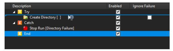
In this example the Action will be dropped After the action above the line, because the guide line indicators point up.
