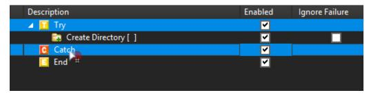
In this example the Action will be dropped Before the action under the guide line, because the guide line indicators point down.
