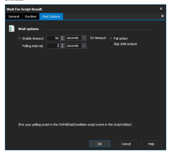
In this example the FinalBuilder variable MyCounter is incremented by 2 and then evaluated to see if the value is greater or equal to 10. If the value is less than 10 then the action will poll again after the specified period (set via the Wait Options tab of the action).
