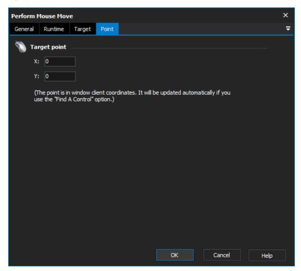
Choose the target point for the mouse to move over. The point is in client coordinates of the control window.
