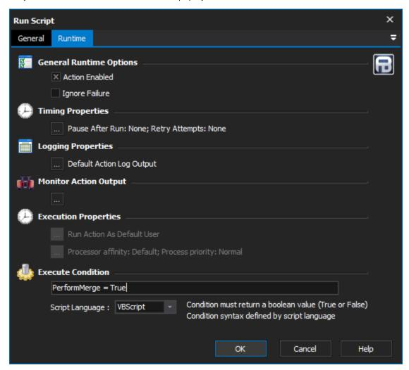
The Execute Condition field is evaluated before running the action. If the condition evaluates to True (or is empty) then the action will execute, otherwise the action will be skipped.
