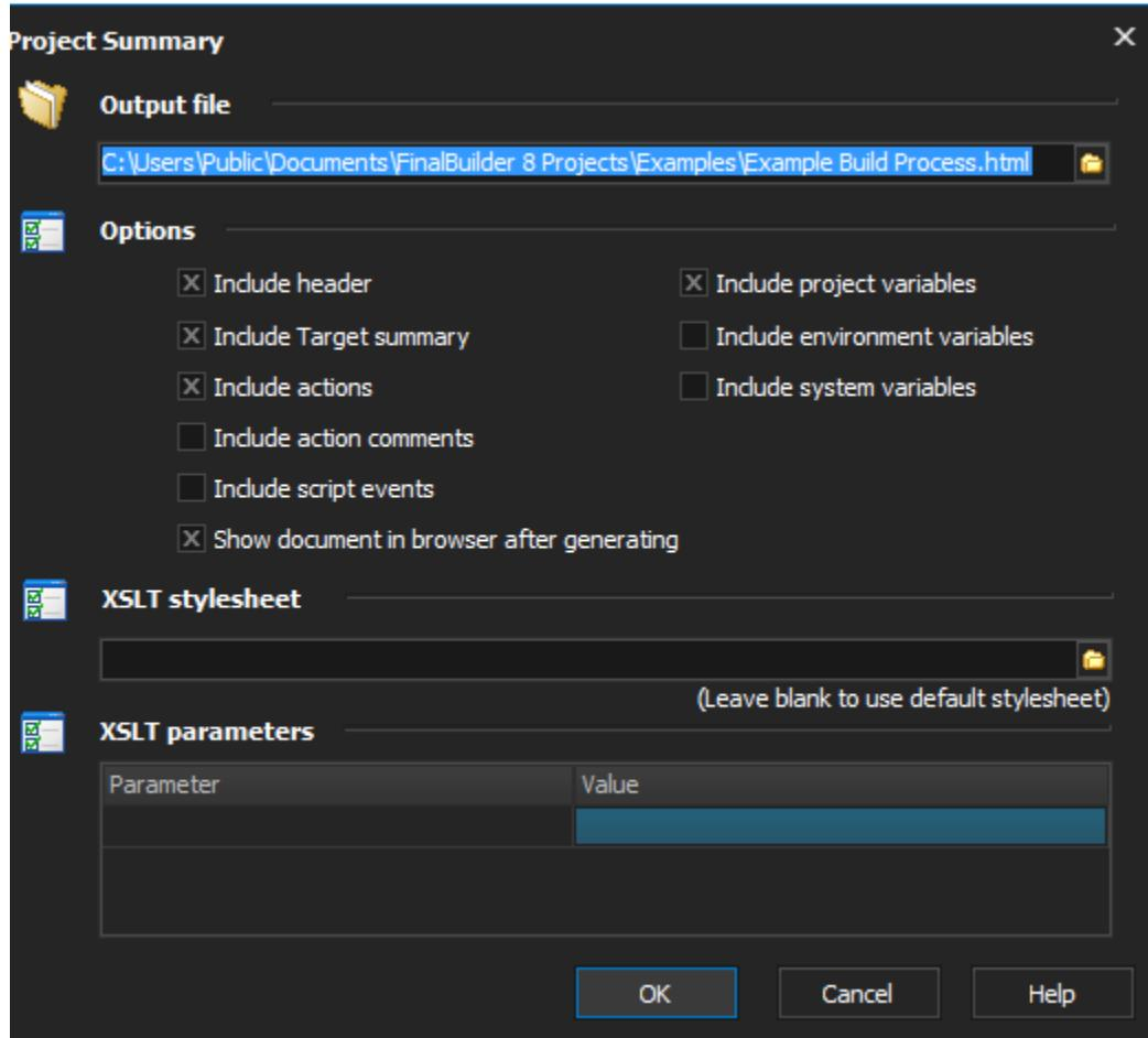
The XSLT stylesheet option allows you to use your own custom stylesheet to control the format of the output. If this field is left blank the default stylesheet (<install\_directory>\Stylesheets\CreateProjectSummaryFromProject.xsl) will be used.
